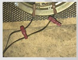
Insert the wires from the PINsub MS into the hole in the small endcaps. Carefully twist the small endcaps until finger tight.
