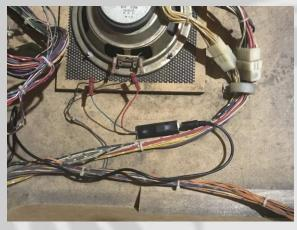
Locate the vent hole in the right rear of the cabinet. Push up on the vent screen to dislocate it to allow the 3.5 mm cable to be fed down through the vent hole.
