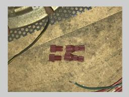
Place the large endcaps over one of the two speaker wires.
