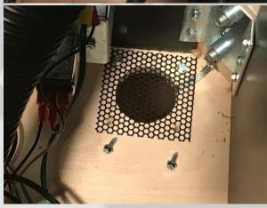
Fish the 3.5mm subwoofer cable through the vent hole in the bottom of the cabinet.
