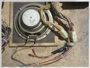
Remove the two PosiTaps by twisting the smaller end cap.
