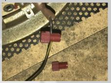
Twist the middle section back on to the larger endcap. Finger tighten but don't force it.
