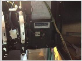
Move the nylon cable clamp to the front of the spacer used in the upper right corner of the plate. Fasten with the original hardware.
