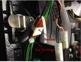
Insert the PP2MAC cable connector into the two female connectors as shown below.
