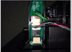
Make sure that the JJPMAC cable is routed under the coin mechs. Wrap the wire and tuck it into the area shown.
