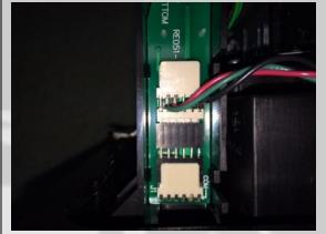
Insert the original cable into the JJPMAC connector.
