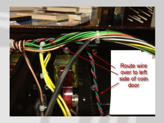
Cut the tie-wrap as shown then disconnect the male to male jumper.
